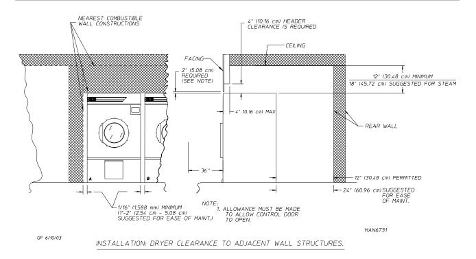
**NOTE:** When fire sprinkler systems are located above the dryers, a minimum of 18-inches (45.72 cm) above the dryer console (module) is required. Dryers may be positioned sidewall to sidewall, however, 1 or 2-inches (2.54 or 5.08 cm) is suggested for ease of installation and maintenance. Allowances *must be* made for the opening and closing of the control door and the lint door.
